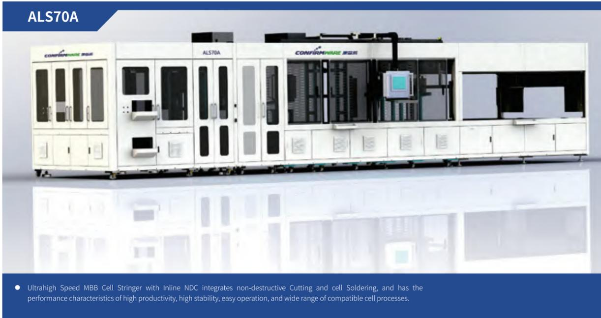
● Ultrahigh Speed MBB Cell Stringer with Inline NDC integrates non-destructive Cutting and cell Soldering, and has the performance characteristics of high productivity, high stability, easy operation, and wide range of compatible cell processes.
